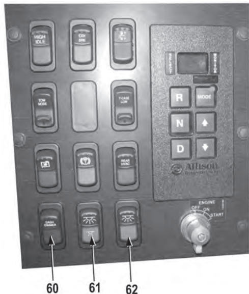
Figure 2. Instrument Panel Controls and Indicators (Sheet 12 of 16).
